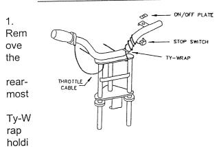
the Twist Grip (REF 47) and Stop Switch (REF 14) secure during shipping. Discard the Ty-Wrap. Also remove the Ty-Wrap holding the two Handlebar Grips together. Discard the Ty-Wrap. Slide the Dummy Grip (REF 49) onto the Left Handlebar (REF 50).
