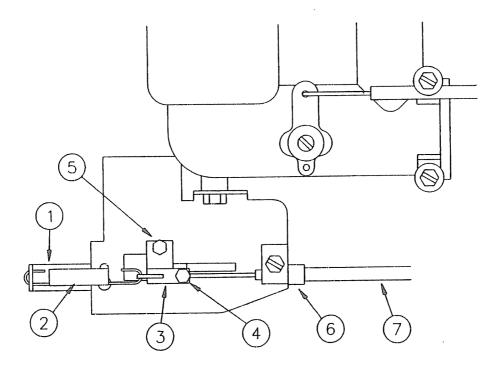
Throttle Cable Installation: Pass the Throttle Cable through the Throttle Cable Retainer (Ref. 6) and butt the end of the Throttle Cable Housing against the inside shoulder of the Throttle Cable Retainer. Pass the end of the Throttle Cable through the Cable Stop (Ref. 3).
