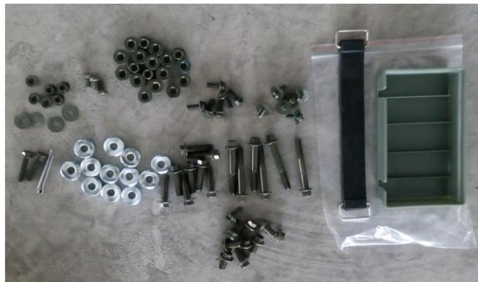
1.4.3 Bag 3: Steering wheel cover (1pc), cable for headlight (1pc), clamps for windshield (10pc), clamp cushion for windshield (4pc), plastic plug (2pc), self-locking nut M10X1.25 (2pc), bolt M5X25 (1pc), washer  $\phi$  5 (1pc), rear mirror mount and O-ring (1pc)
