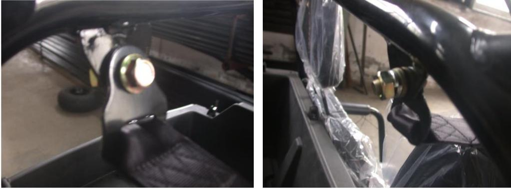
2.15 Install the seat back head rest (No this step with new sport seat!)
